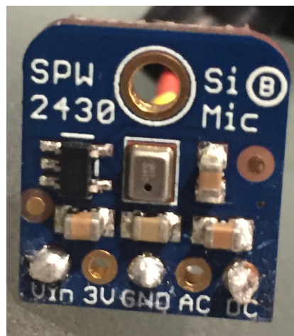
Figure 4.12: Adafruit Silicon MEMS Microphone Breakout-SPW2430
