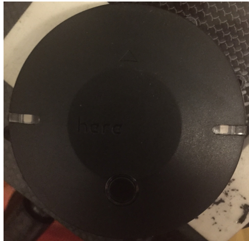
Figure 4.11: HERE Solo GPS Module
