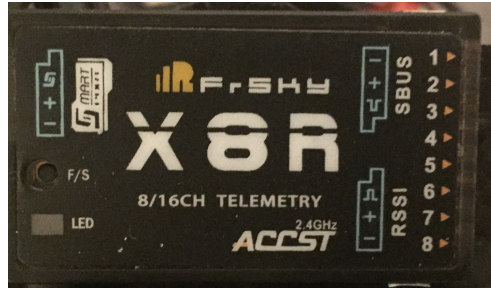
Figure 4.10: FrSKY X8R 2.4GHz Receiver
