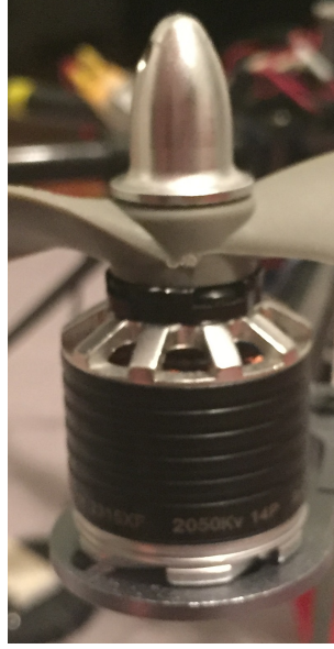
Figure 4.2: KDE 2315XF-2050 Motor
