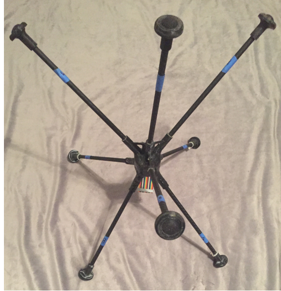
Figure 4.13: 8 Channel Microphone Array Design
